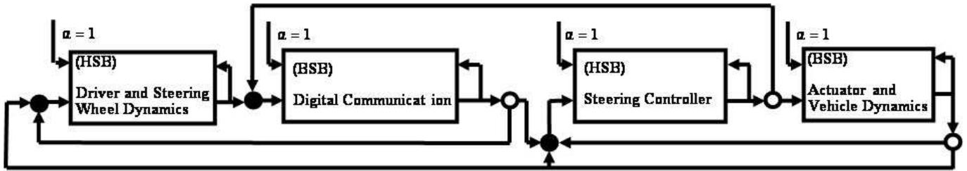
Figure 10. Reduced order Steer-by-wire system block diagram (top level).
