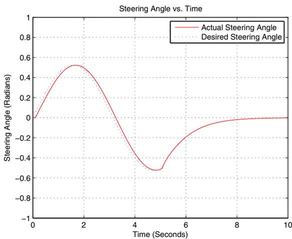
**Figure 19.** Steer-by-wire simulation (human mode switching at  $t = 5$  seconds).
