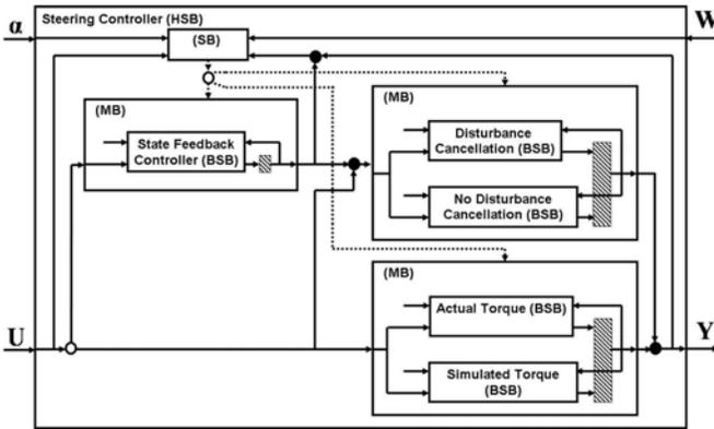
Figure 9. Steering controller block diagram (In all Figures, dotted lines represent the SB block output).
