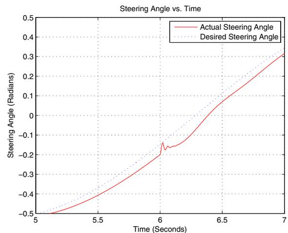
**Figure 18.** Steer-by-wire system simulation (torque sensor failure at  $t = 6$  seconds).
