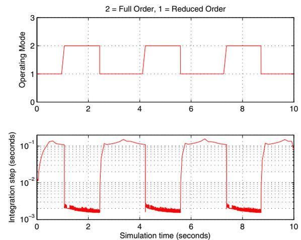
**Figure 21.** Model order switching and integration step vs. simulation time (step size ratio = 1:50).
