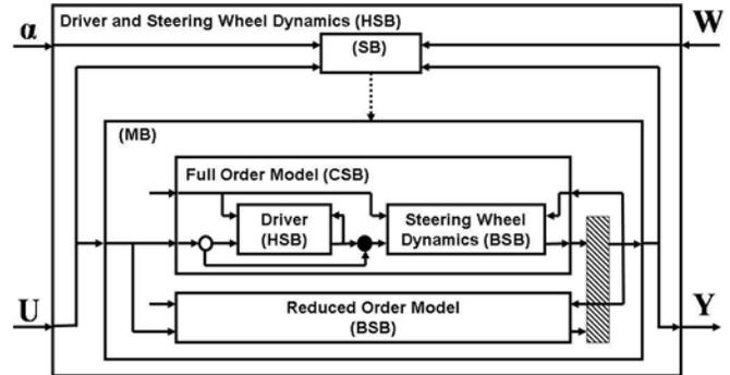
Figure 11. HSB containing both full-order and reduced-order models for driver and steering wheel.
