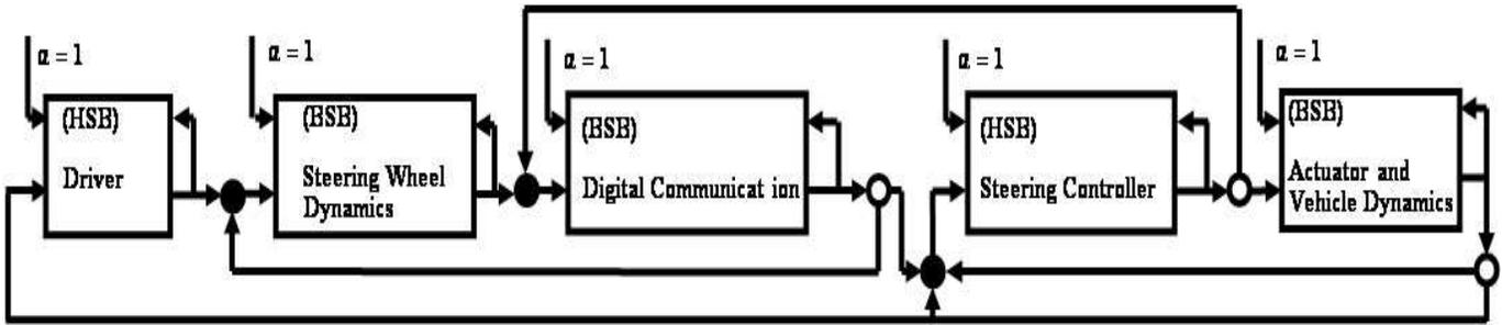
Figure 7. Steer-by-wire system block diagram.
