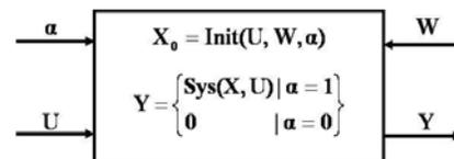
**Figure 1.** Basic system block (BSB).
