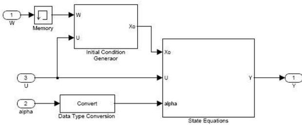
Figure 12. Simulink implementation of a BSB.
