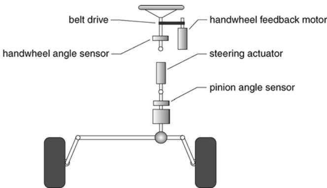
Figure 6. Steer-by-wire system (from [10]).
