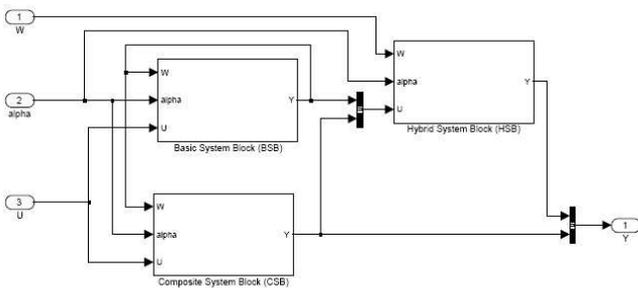
Figure 13. Simulink implementation of a CSB.
