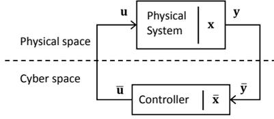
Figure 1: A System Diagram of CPS.
