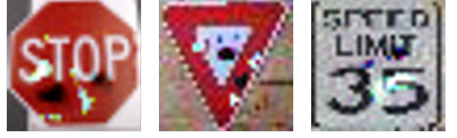
Figure 3: Perturbation generated by the RP_2 attack using the authors-provided code under the \ell_1 norm so that a stop, yield, and speed limit 35 sign are misclassified by the LISA CNN [3] as speed limit 35, speed limit 35, and turn right sign, respectively.
