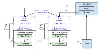
Figure 4: Block diagram of the framework and ADS (in blue) integrated into the hierarchical system
