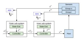
Figure 3: Block diagram of the hierarchical system
